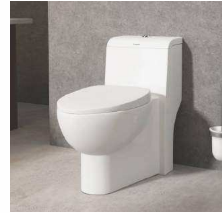
NOVA One Piece EWC - 42010BS/P Soft Close Seat Cover - 43010S Dual Flush - 45010 L720 W377 H730mm Wash Down Flushing, 'S' Trap 230mm, 'P' Trap 180mm
